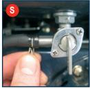
Refill the tank with fuel and ensure there are no leaks between the tap and the tank, and with the fuel tap turned on, ensure there are no leaks where the fuel hose is fitted to the outlet of the tap.
